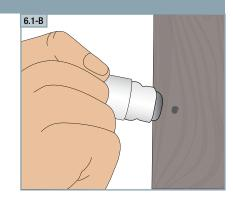
Touch-up Pens - conceal nailheads and very small nicks and scratches less than a dime size. Replace the area with a new piece of plank or panel if area is larger than a dime.
