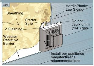
For dryer vents, avoid placement too low to the ground where debris could easily impede air flow, trapping heat and moisture. Some types of high efficiency furnaces can be vented out through the walls. In these cases, avoid locating the vent too close to the roof or eaves where heat and moisture will be trapped.
