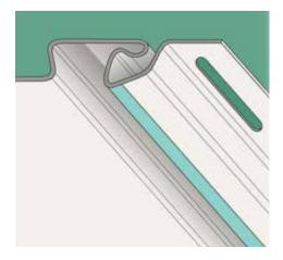
Charter Oak soffit is one of the most rigid soffit products on the market. Its superior rigidity is the result of Alside's exclusive TriBeam system. The result is a panel that's not only stiffer than competitive panels, but also lighter and easier to install.
