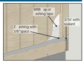
Sheathing Framing-Nail into WRB framing
