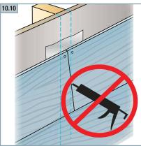
Caulking at HardiePlank lap siding butt joints is not recommended for ColorPlus for aesthetic reasons as the caulking and ColorPlus will weather differently. For the same reason, do not caulk exposed nail heads. Refer to the ColorPlus touch-up section for details
