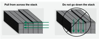
TIP: When taking planks from the pallet installation, avoid repeating the texture pattern by working across the pallet. Two to four planks can be removed from a stack at one time. But then material should be taken from adjacent stacks, again working across the pallet. Texture repeat is typically a concern on large walls with few breaks such as windows or doors.
