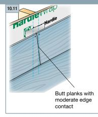
COLORPLUS® TIP: When installing HardiePlank lap siding with ColorPlus Technology, position the plank in the immediate area where the plank is to be fastened. Do not place the plank on the course below and slide into position. Doing so may scuff or scratch the ColorPlus finish on the installed piece.
